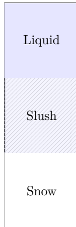
Figure 5: Illustration of melting process, going from frozen snow, to a slush region and finally a fully melted water film.
